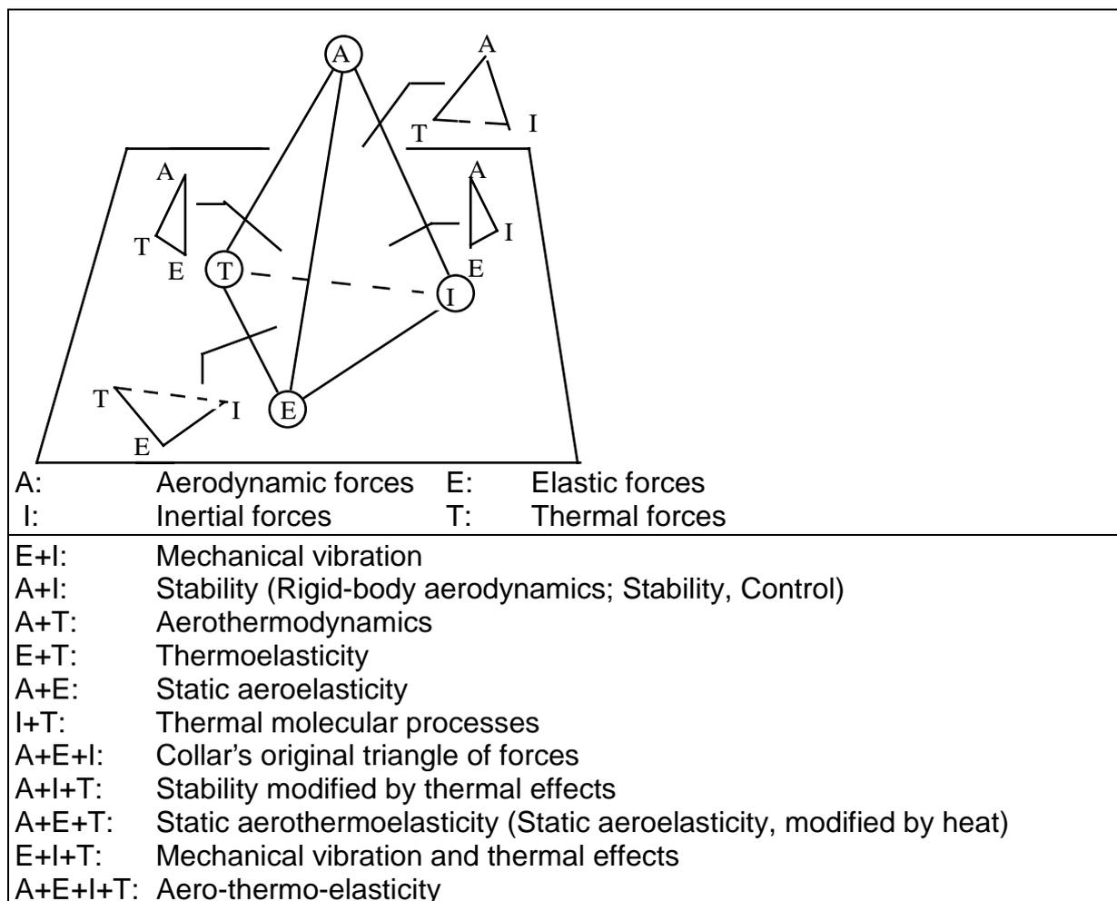
**Fig. B1C1.5:** Tetrahedron of aerodynamic, inertia, elastic and thermal forces [Garrick, 1963, p. 130].
