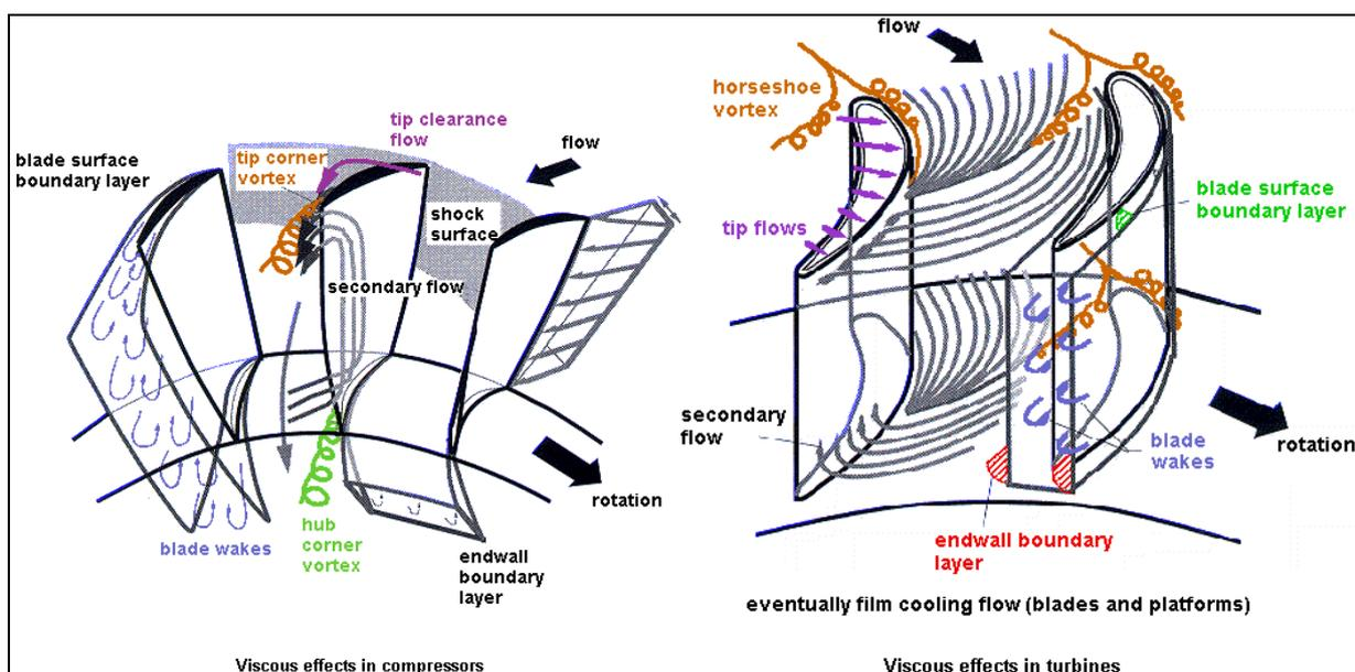
**Fig. B1C1.6:** Rotor blade row phenomena [Compressor figure originally from McNally, 1977, p. 458]
