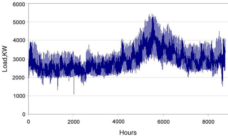
Fig. 4. Hourly average electricity system load, 2000.
