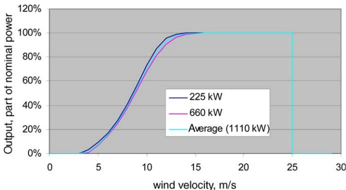
Fig. 1. Porto Santo installed Vestas wind turbine characteristics.
