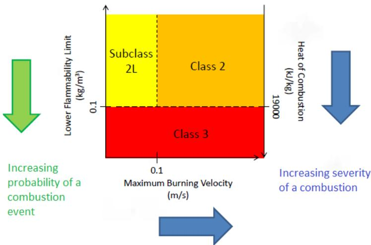
Figure 3 - Flammability classes of flammable refrigerants according to ASHRAE standard 34
