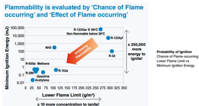
Figure 1 - Minimum ignition energy and lower flame limit for selected refrigerants
