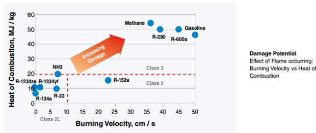
Figure 2 - Heat of combustion and burning velocity for selected refrigerants
