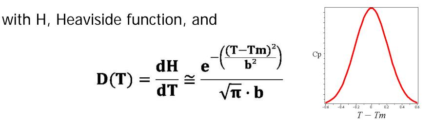
parameters are chosen to account for 1K phase change temperature range with latent heat peaking at phase change point
