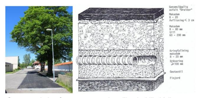
System solution for storm water handling in *Lilla Vallen, Växjö*. The road system consists of drainage asphalt. (Sörelius et al., 2017).
