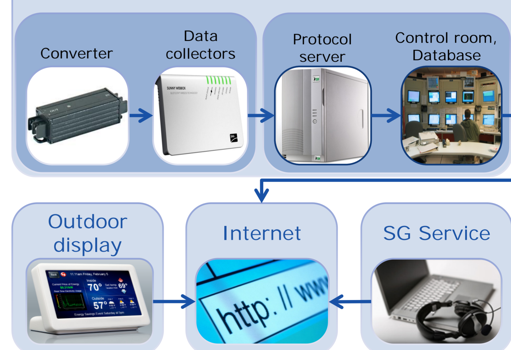
Fig. 6: Architecture of the communication package
