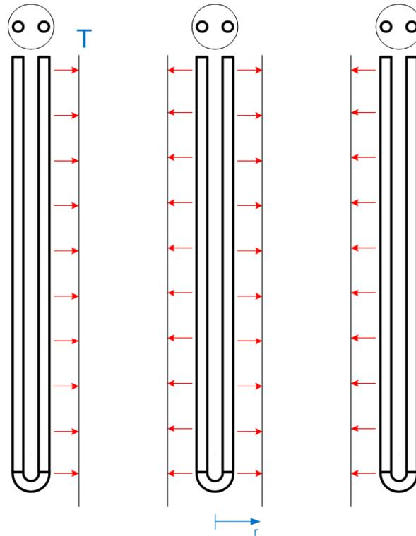
Obtained using the cylindrical heat source analytical solution
