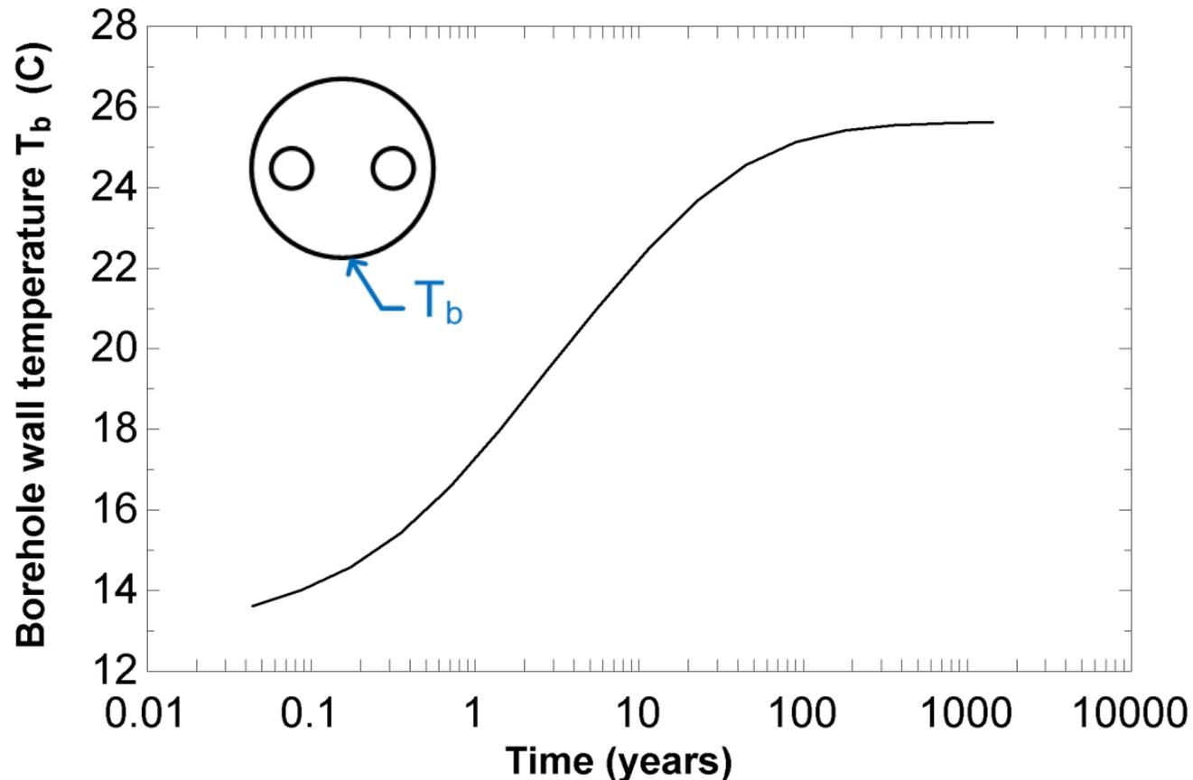
Curve shown is only valid for a particular geometry and ground temperature
