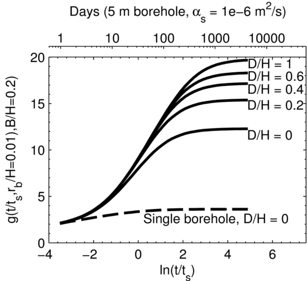
**$6 \times 4$  bore field with  $H = 5 \text{ m}$ ,  $B = 1 \text{ m}$ , and  $r_b = 0.05 \text{ m}$**
