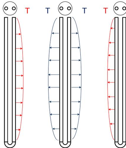
2-D heat transfer and borehole thermal influence not accounted for
