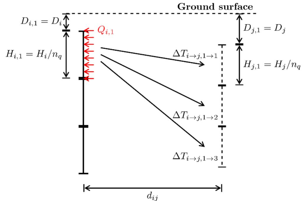
Analytically using the Finite Line Source solution (see Cimmino and Bernier, 2014)
