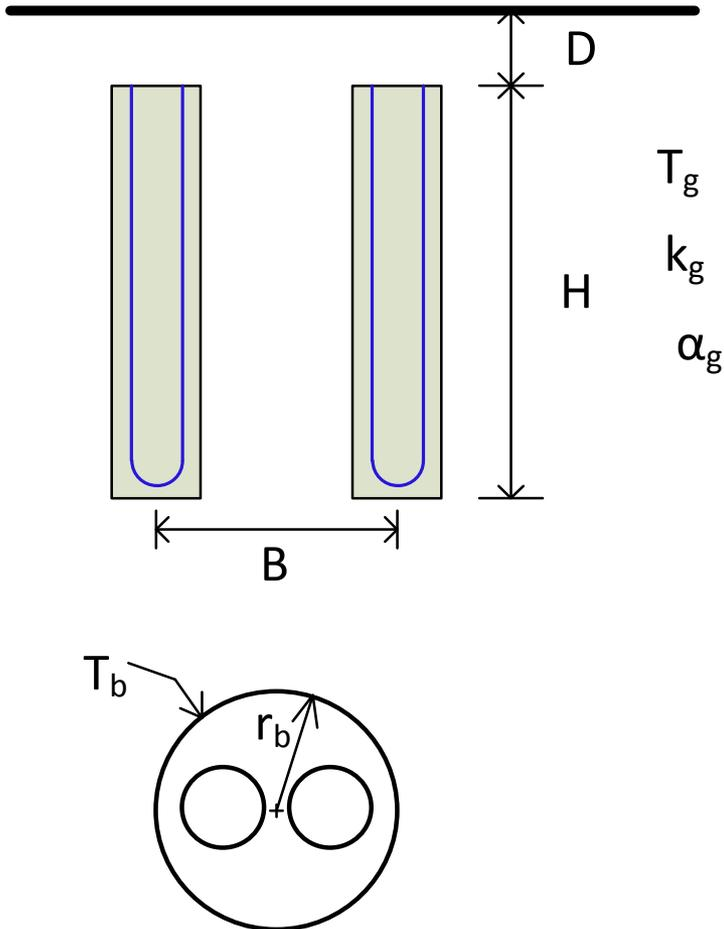
Eskilson determined that for a given bore field geometry and for deep boreholes, the thermal response of a bore field depends on 3 non-dimensional parameters:
