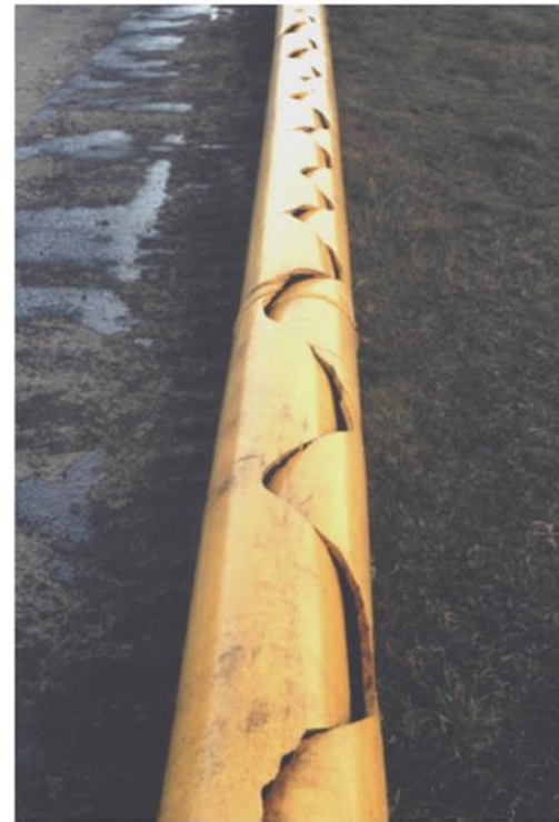
Rapid crack propagation in 315 mm SDR 17 PE80 pipe
